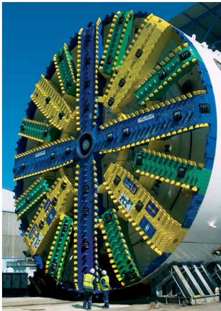
TBM for enlarging the M-30. Madrid
