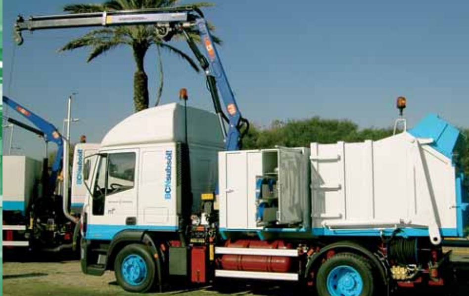
Solid urban waste collection vehicle that runs on compressed natural gas
